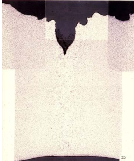
Figure 9. Selective seam weld corrosion viewed in cross section
